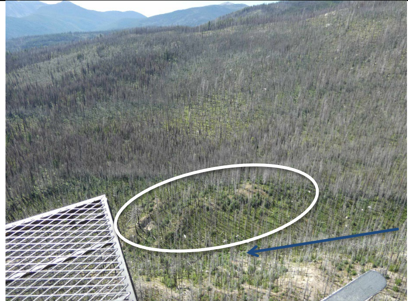
Photo 2: Burned headwaters of Shoudy Creek and observed terrain instability (circled) along incised reaches. Note, channel is visible at the bottom of photo (arrow).
