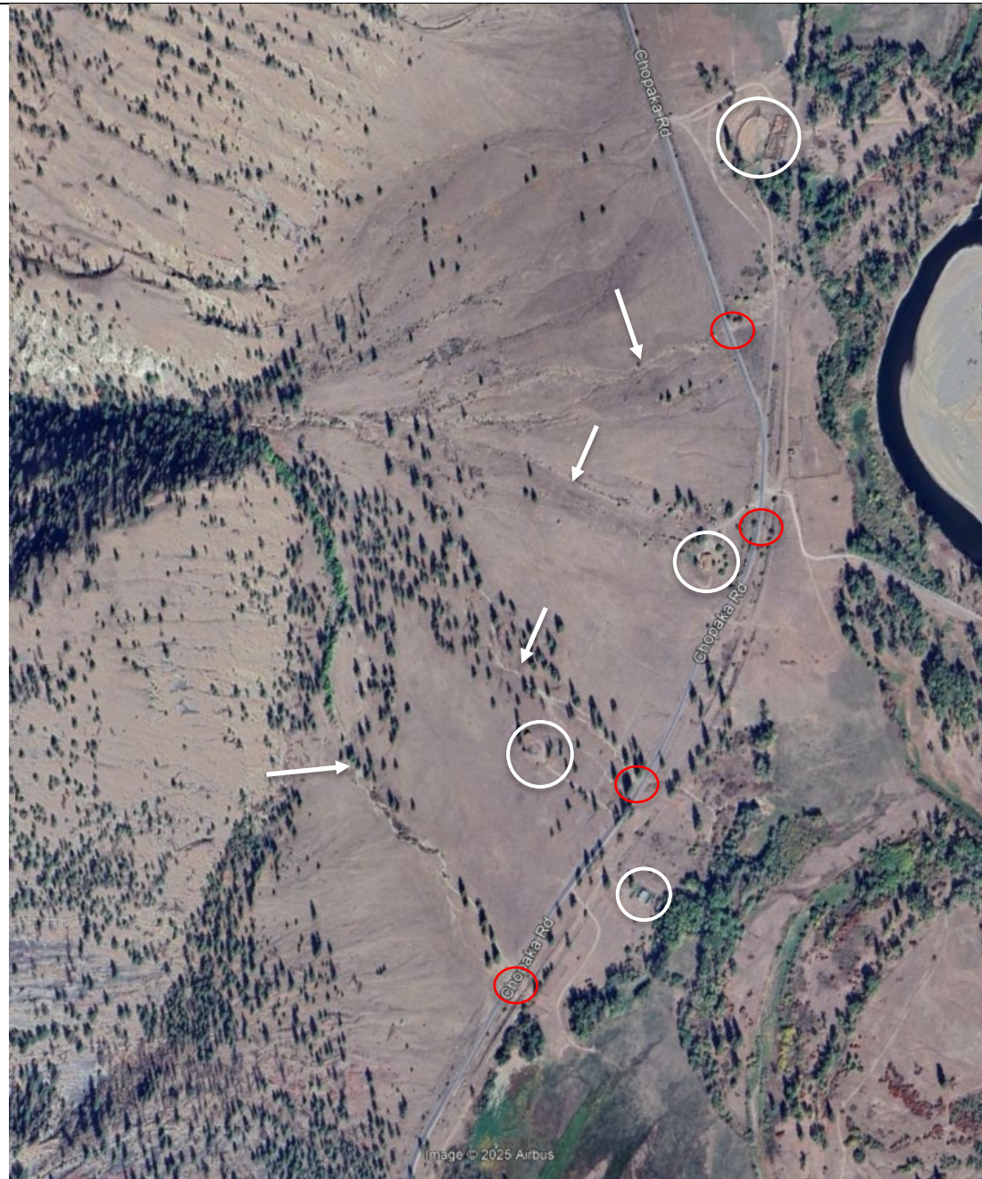
Photo 5: Shoudy Creek fan area showing multiple channels (arrows) that experienced recent sediment-laden flooding resulting in impacts to Chopaka Road. Note residences and rodeo grounds (white circles). May 2023 washout locations shown in Photos 6 to 9 are circled in red. Source image from GoogleEarth. See area mapped in Map 002 and Map 003.
