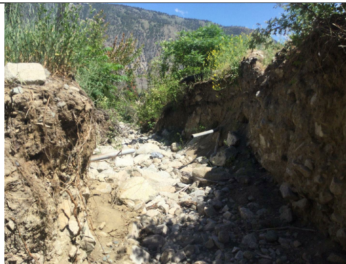
Photo 7: View downstream along dried up channel in upper part of fan. Note deep incision, vertical unconsolidated stream banks, and severed irrigation pipe.
