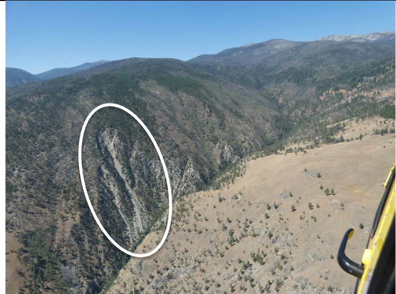
Photo 4: View of large debris slide located ~800 m upstream of Shoudy Creek fan (circled). Recent instability indicated by fresh rock exposure.
