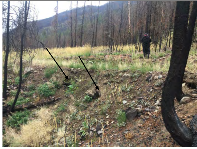
Photo 8: Burn holes (arrows) and deformed trees indicate slope instability along the lower part of Lakeview Road (~1.4 km).
