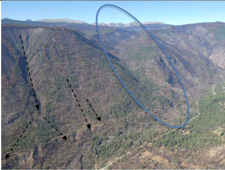
Photo 1: Helicopter overview photo looking south into Lakeview Creek watershed from the Ashnola River (circled). Road on right is Ashnola Road and road on left on terrace is the Lakeview Road accessing Cathedral Park. Note steep, debris-flow prone burned tributaries on Ashnola River Face Unit 4 (arrows).
