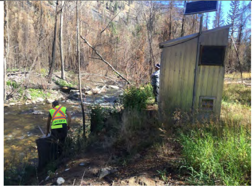
Photo 6: Water Survey of Canada hydrometric monitoring station near the mouth of Ewart Creek.
