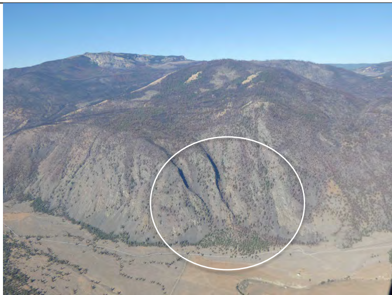
Photo 1: View of Similkameen Sub-Catchments 1 & 2 from the Similkameen River. Note burned areas on plateau, incised bedrock channels & fan area of Sub-Catchment 1 (circled).
