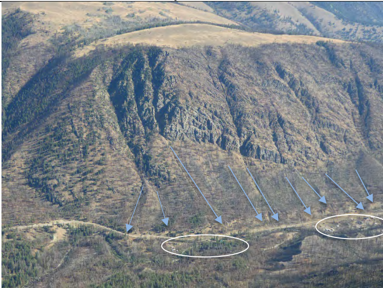
Photo 7: Ashnola Face Unit 3 , east of Meausette Creek. Evidence of multiple post-wildfire runoff flow paths along slopes above Ashnola Road (arrows). Structures/residences and Cathedral Park base camp circled.
