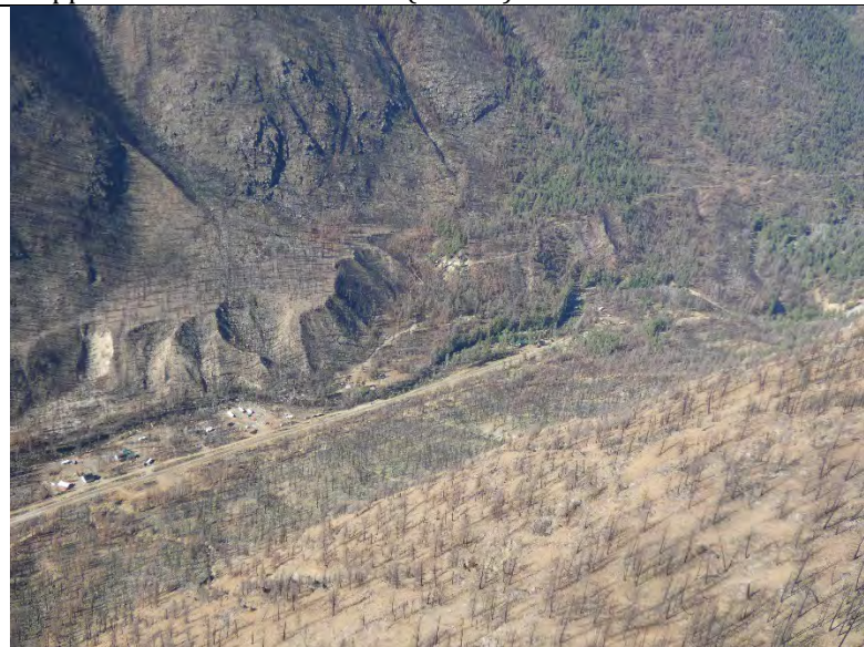
Photo 11: Ashnola Face Unit 4 . Structures/residences and Cathedral Park base camp are visible. Note, large raised fan associated with debris-flow prone catchment and gullied slopes along edge of terrace within the valley.
