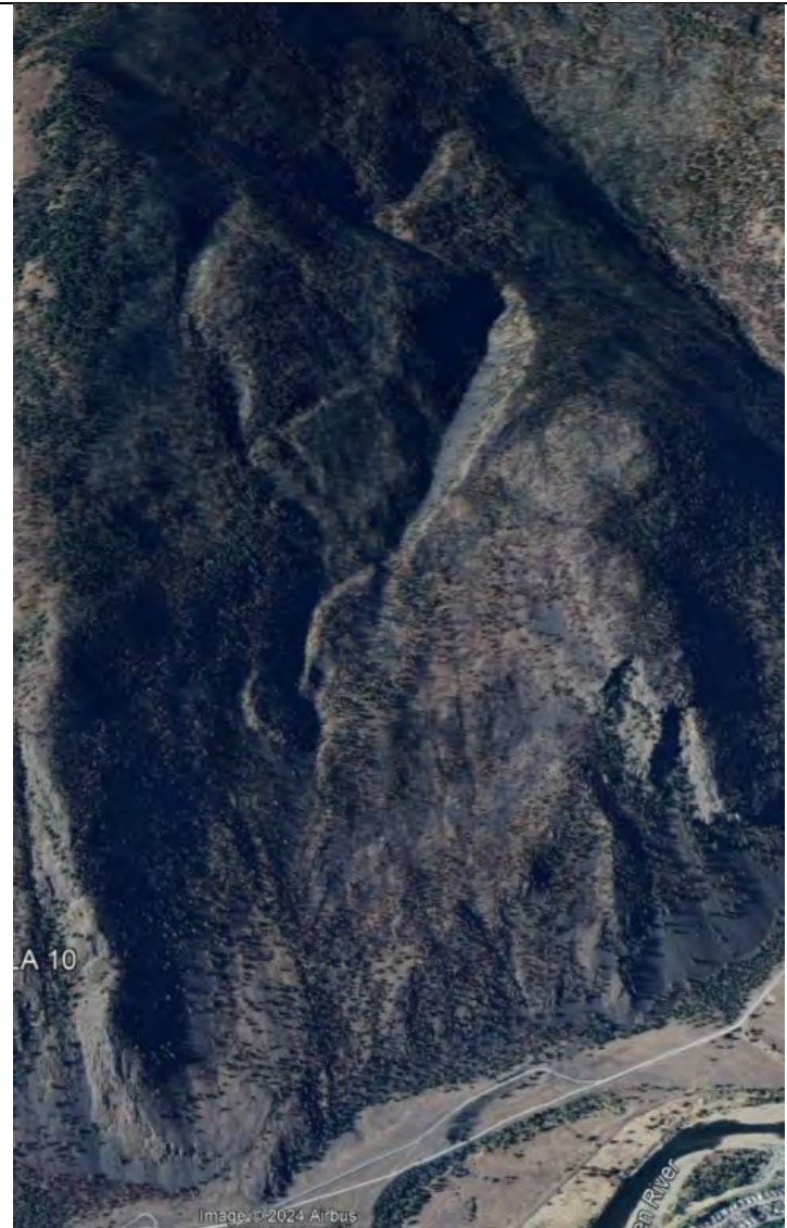
Photo 6: Oblique GoogleEarth image of Similkameen Sub-Catchment 1. Note abundant talus and lack of associated downslope fan (Low Hazard)
