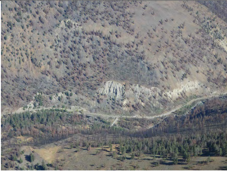
Photo 5: Ashnola Face Unit 2 near Ewart Creek Road bridge. View of west slopes above the Ashnola Road, which are potentially unstable unconsolidated over-steepened glacial drift deposits prone to ravelling (shallow debris slides and rockfall).
