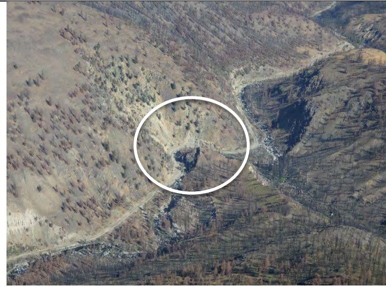
Photo 6: Ashnola Face Unit 3 on the west side of Ashnola River. Photo at confluence of Ewart Creek. Note exposed and ravelling unconsolidated sediments above the road and tight, bedrock-controlled section of valley through which road and river are contained (circled).
