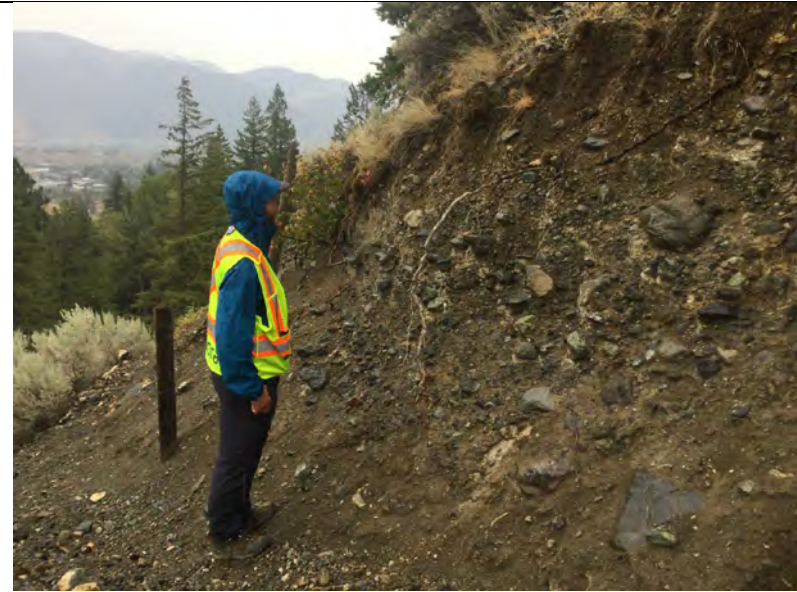
Photo 4: Thin, discontinuous layers of sands and gravels in trail cut on upper part of fan (terrace)
